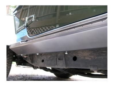
Mask off the area of the car that the rocker will come in contact with including the fender flares. Lift the the rocker into place. Bolt in place using 6 of the 5/16"x1" bolts with a flat washer on each. Hand tighten all of the bolts. Make sure that the rocker is centered on the doors. Once centered tighten the bolts.
