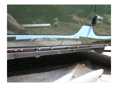
Install the 5/16"x1" bolt with a flat washer thru the rocker support. Tighten the 5/16" nylock with a flat washer on the back side of the pinch weld. When finished you should have 11 5/16" bolts installed and the one factory fender bolt.
